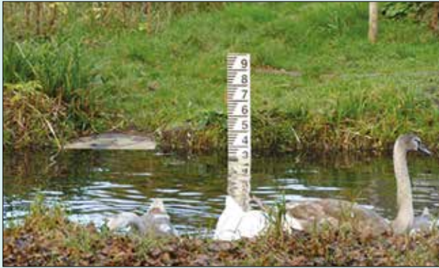
Above: The three gauge boards installed along the Westbrook last winter provide important information for maintaining water levels in our valuable chalk streams. Photo: Matthew Hatchwell.
